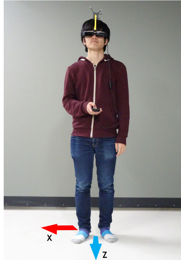
Figure 3. A participant using an OST-HMD with markers for optical 3D motion tracking, having a controller for selection in his hand. Here, he is performing the task with a ray-based technique using IMU.
