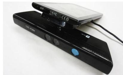
**Figure 4 - CrashAlert prototype: Acer A100 + Kinect.**
